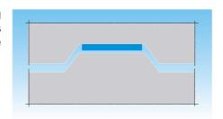
The applied profile is chosen so that the elements create already at assembling a pre-stress. A proper plugging by means of mounting cements like *F60 / F300* or permanently elastic sealants e.g. *FIX-O-FLEX H* or *FIX-O-FLEX VG* can be achieved.
